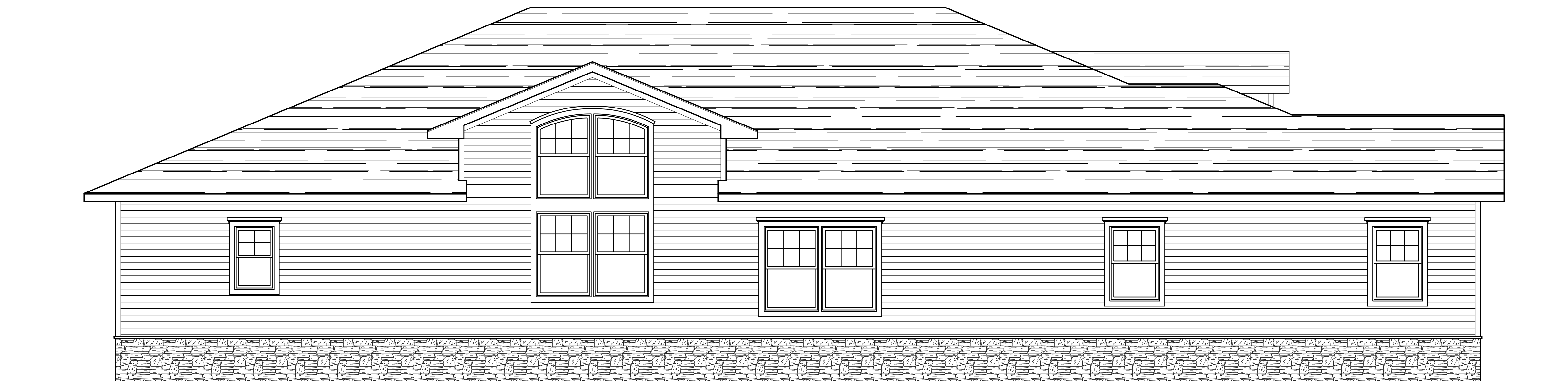
SIDE (WEST) ELEVATION SCALE: 1/4" = 1'-0"
